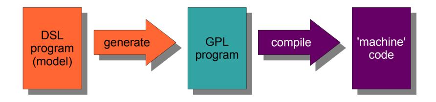
raise the level of abstraction to a technical or application domain *automatically* generate implementation code from model
